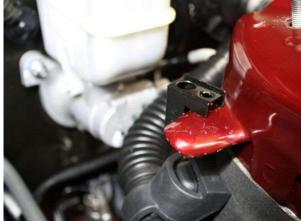
Use the supplied  $\frac{1}{2}$ -20x $\frac{1}{2}$ " bolt and attach J&L Bracket to the black mounting clamp using the smaller hole as shown below:
